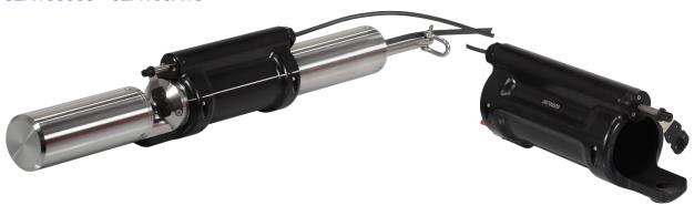
The TriOS Wiper W55 V2 provides an additional cleaning option for all TriOS photometers with path lengths from 1 mm up to 10 mm. The wiper housing can be mounted on the sensor in just a few steps and provides reliable cleaning of the measurement windows. The new magnetic axis lock allows quick and easy wiper blade replacement, without any tools.
