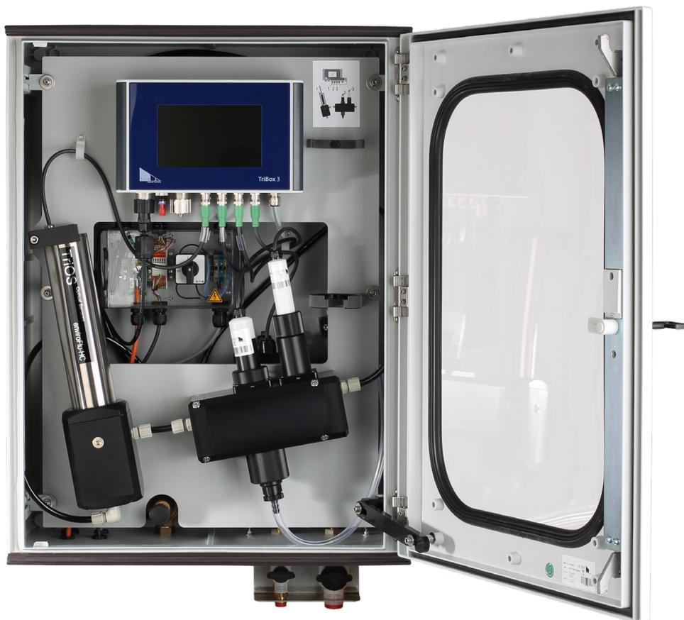
The EGC Water Analyzer is TriOS' latest development in the monitoring of various wastewater-parameters. It can be equipped with three sensors: enviroFlu for identification of polycyclic aromatic hydrocarbons (PAH), TTurb for turbidity measurements and TpH-D for the determination of the pH value.
