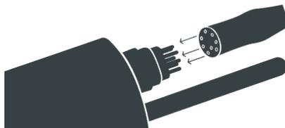
The next step is to rotate the locking sleeve in a clockwise direction to lock the end of the connector into the bulkhead connection.
