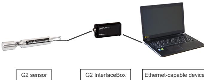
The TriOS G2 InterfaceBox translates the 8-pin M12 sensor plug to the conventional power supply connections (2.1 mm barrel connector) and to the network access (RJ45 socket).
