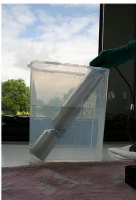
The zero value of the LISA UV is checked via the web interface. To access the web interface, you will need the G2 InterfaceBox and an Ethernet-capable device with a web browser, such as a notebook / laptop.
