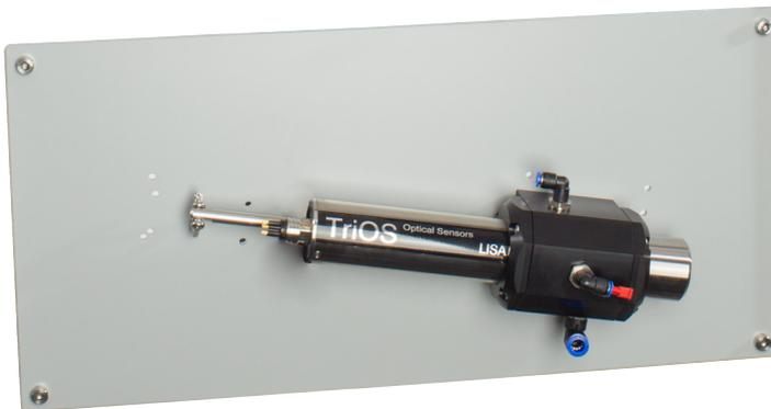
**NOTICE** The maximum pressure in the flow cell must not exceed 1 bar. Make sure that the sensor is installed in the correct position to guarantee the free flow of water.
