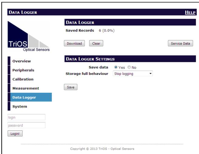
The previously stored data can be retrieved by clicking on the “Download” button. The sensor presents this data as a CSV (comma-separated values) file, which can be read by conventional spreadsheet programs.
