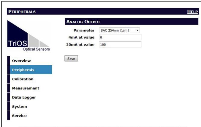
The “analog” version offers three options on the “Peripherals” page of the web interface: the parameter to be output as well as the lower and upper limits for the linear spread of the measurement value from 4 mA to 20 mA.
