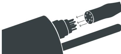
The next step is to hand-tighten the locking sleeve to secure the end of the connector into the bulkhead connection.
