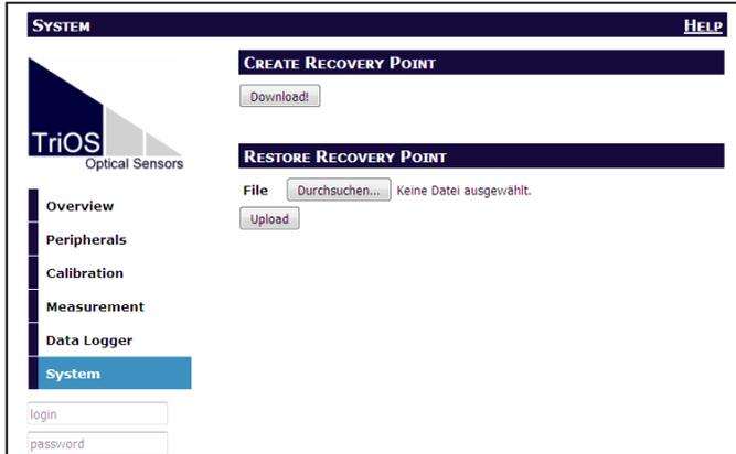
By clicking on the “Download” button, the current calibration of the sensor can be downloaded and saved, for example, on a PC. The LISA UV presents all relevant data in the form of a calibration file, as can be seen in the figure below. This file must be stored and kept safe.
