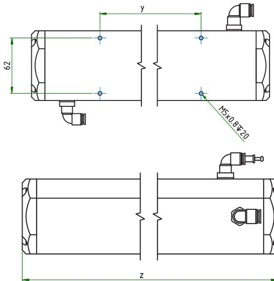
The hoses are installed by putting light pressure on the hose connectors. To remove the hoses, press on the locking ring on the hose connector and carefully pull the hose away.
