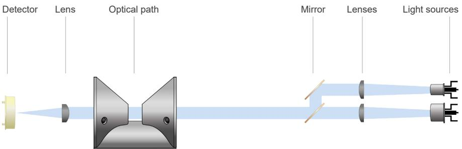
LISA UV essentially consists of four parts: a defined light source, a lens system, the optical path through the medium and a detector with ambient light suppression. The arrangement of these parts is represented schematically in the above illustration.
