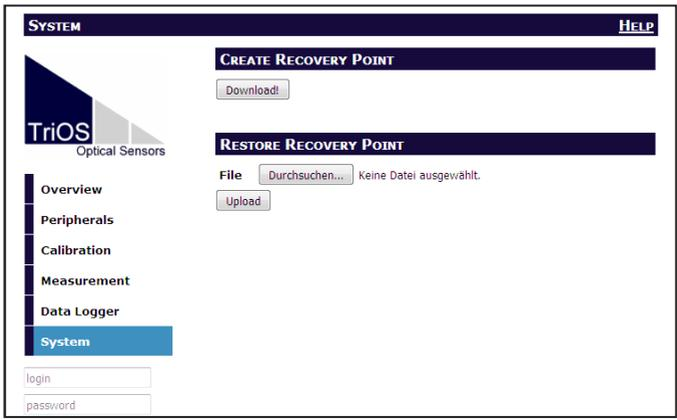
Enter the storage path for the appropriate calibration file in the “File” field or select it with the help of the file dialogue by clicking on the “Browse...” button. Next, click on the “Upload” button to begin the transfer. When the process has been successfully completed, this will be indicated by a green “Success” box. If the process is not successful, a red box will be displayed with an error message.
