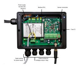
Pin Assignment 1 RS-485 A 2 RS-485 B 3 Ground
