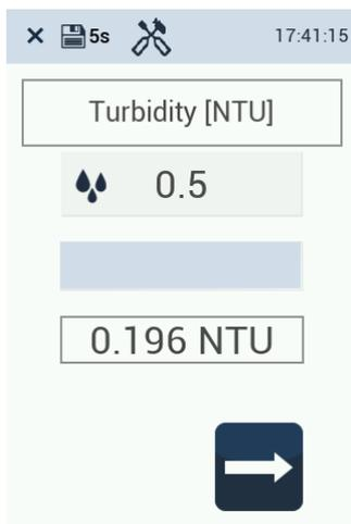
When the calibration is complete, the arrow at the bottom right of the display is activated. Click on this button to check the calibration.
