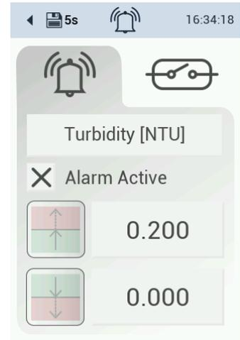
The relay can be set in the same way. To change the values, click on the values. To activate the functions, click on the checkbox.
