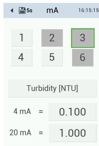
The analog output being configured is outlined in green. Outputs that are occupied are highlighted in gray. Outputs assigned by another device must first be enabled before they can be assigned again.
