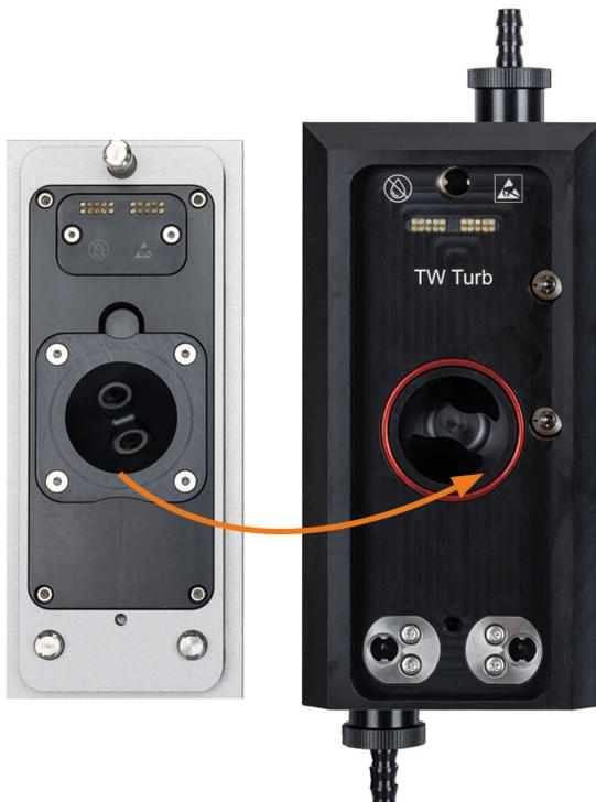
The sensor measures according to the nephelometric principle of 90° infrared scattering. The scattering intensity measured by the detector, which is positioned at a 90° angle to the light source, can be used to precisely determine the turbidity of a liquid.
