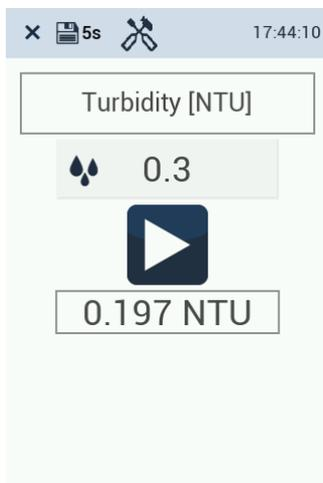
The sensor now begins to stabilize the value. When the sensor is ready, click on the “Play” button. The sensor starts the calibration process.
