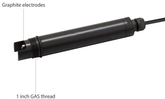
The conductive measuring sensor has two graphite electrodes facing each other. A voltage is applied to the electrodes so that a current is generated in the measuring medium.
