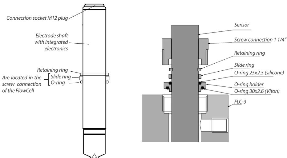
5. Carefully slide the previously unscrewed 1 ¼" screw connection over the sensor inserted in the fitting and screw tight, otherwise leaks may occur!
