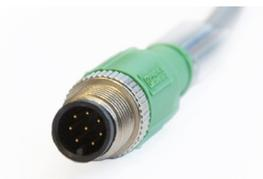
Insert the connector into one of the supplied TriOS cables (2 m). Additional cable lengths of 0.3 m, 2 m, 5 m, 10 m, 25 m are offered. Connect the male end of the cable into the connector on the sensor by making the pins align with the slots of the cable. The next step is to turn the locking sleeve clockwise to secure the end of the connector.
