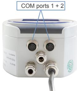
The TriBox mini has two M12 sensor interfaces, which can also be used as digital outputs. The sensor interfaces support RS232 and RS485 and can be configured for Modbus.
