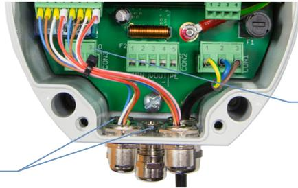
Cable bushing for a relay
