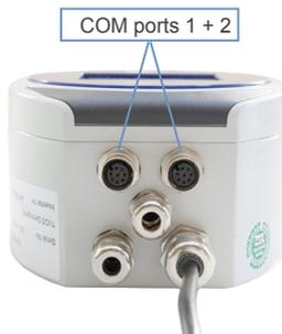
Both M12 sensor interfaces support RS232 and RS485 and can be configured for Modbus and other special protocols.
