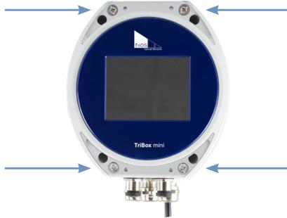
3. After removing the four screws, carefully lift open the cover of the housing. The housing cover should open without resistance and without application of force, as this would present the risk of damaging conductors in the device.
