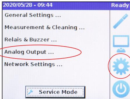
The parameters and resolution can be customised and configured. The analog signal can be fed to external systems, such as PLCs and SCADA, to be transformed into measurement signals. The minimum is 4 mA; the maximum is 20 mA.
