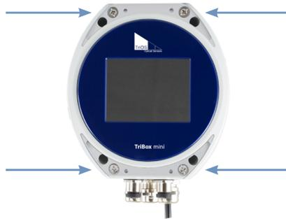
3. After removing the four screws, carefully lift open the cover of the housing. The housing cover should open without resistance and without application of force, as this would present the risk of damaging conductors in the device.
