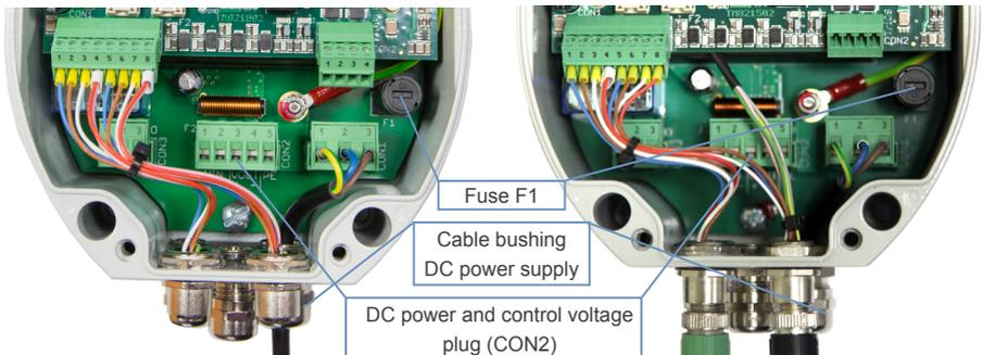
5. Insert the plug back into the socket and tighten the grommet to achieve a solid yet not excessively tight seat of the supply line in the grommet.
