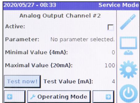
To configure an analog output, it must first be activated ("Active" check mark). Next, a parameter must be selected. To do this, tap the "Parameter" field on the display. In the last step, the values are defined to connect the configuration of the analog output.
