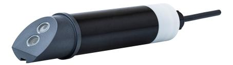
The TTurb is a digital sensor for optical turbidity measurement using the 90° IR scattered light method. Depending on the sensor version, it can be used in pure water up to 100 FNU as well as in raw water, waste water and process water up to 1000 FNU. TTurb is available with different cable lengths (10 m, 2 m or 0.5 m) and in different versions.
