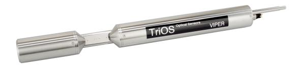
VIPER measures the spectrally resolved light attenuation in the wavelength range from 360 to 720 nm and thus enables the simultaneous, precise determination of several parameters. Five selected, energy-saving LEDs serve as the light source and ensure stable measurement results and a long service life.
