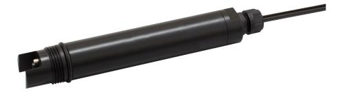
Conductivity sensors are measuring devices that measure the ability of a medium to conduct electrical current between two electrodes. The current flow takes place through the transport of ions - the higher the concentration of charged particles in the medium, the better it can conduct electricity.
